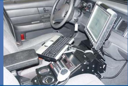
MW800 Swivel Monitor Mount (S-UMM-MOT-M80)
