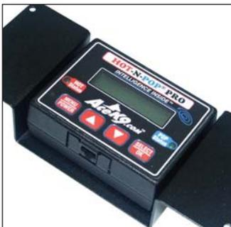
**AceK9® Remote Door Popper and Heat Sensor Unit** alerts the officer when car temperature is too high. Will drop windows and turn optional exhaust fan on. Comes standard with key fob door popper to allow K9 to come to officer aid in seconds. (KK-K9-HP-5010-H) Pager alert and other option available.
