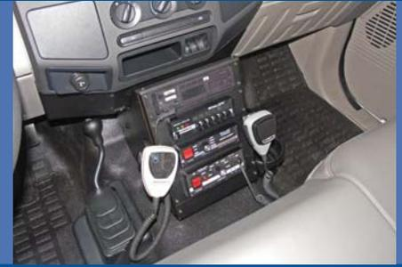
Console Installed in Ford F-250 (C-VS-1200-F250-1)
