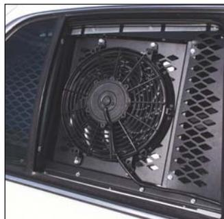
**Heavy-Duty Exhaust Fan** quickly circulates air inside the car (KK-K9-FKT-I mounted on KK-K9-FAN-F7-1-OBR)
