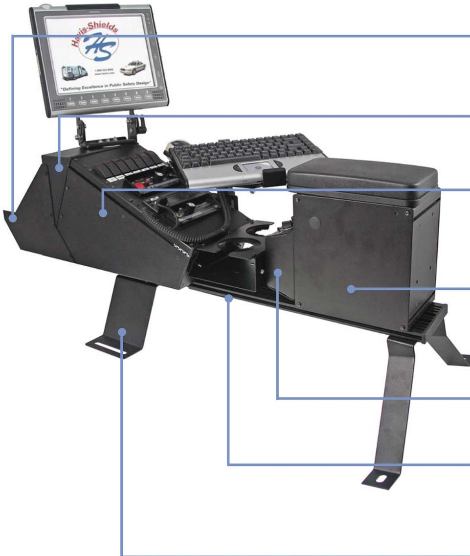
**Wire Cover Panels** provide a nice flush fit to your dash creating the perfect finishing touch and protecting console wiring (C-AS-WP-CV shown)
