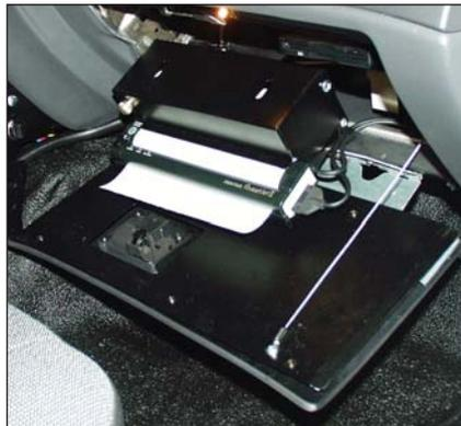
Glove Box Printer Mount (C-3610-CV)
