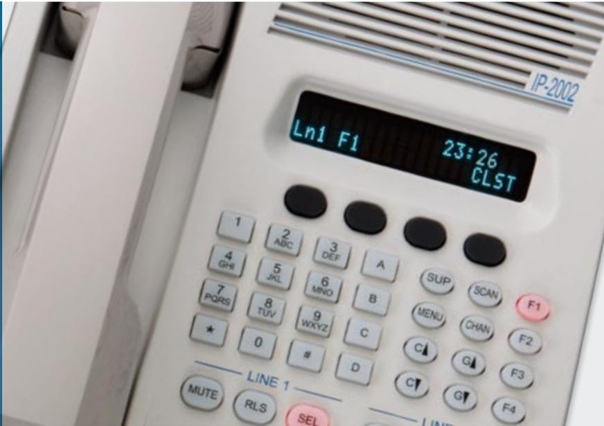
The perfect footprint for smaller operations or supervisory monitoring situations, the IP-2002 is an IP-based dispatch console in a familiar desktop telephone form factor. Dispatchers using the IP-2002 can initiate a crosspatch between the two lines as well as inject audio into the crosspatch. A simple Ethernet connection
